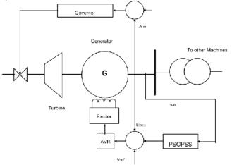
Fig. 2. Single Machine Infinite Bus System.
