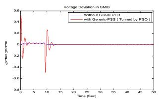
Fig. 6. Voltage deviation without PSS & with PSO based PSS fault at  $t = 5 \text{ sec } (\Delta T = 0.05 \text{ p.u}).$
