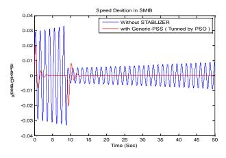
Fig. 4. Speed deviation without PSS & with PSO based PSS fault at  $t = 5 \sec (\Delta T = 0.05p.u)$ .
