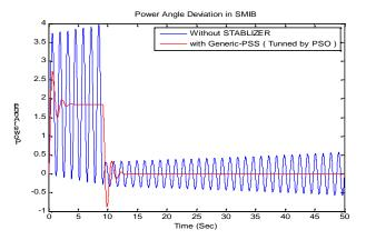
Fig. 5. Power Angle without PSS & with PSO based PSS fault at  $t = 5 \text{ sec } (\Delta T = 0.05 \text{ p.u}).$
