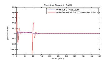
**Fig.7.** Electrical Torque without PSS & with PSO based PSS fault at  $t = 5 \sec (\Delta T = 0.05p.u)$ .
